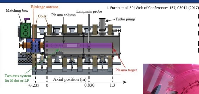
Helicon plasma discharge on RAID (EPFL) RF power 3-5 kW, pressure 0.3 Pa, Magnetic field: 10 mT
