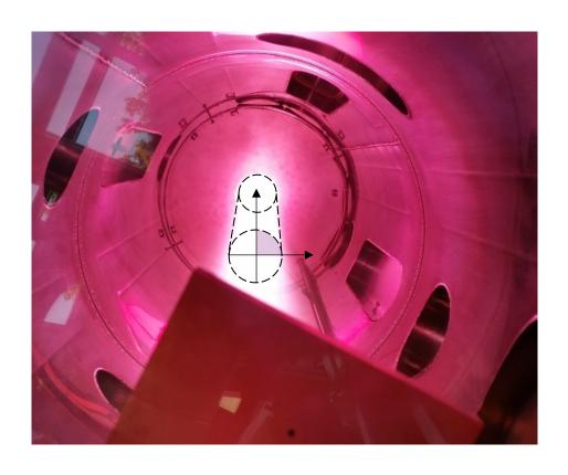
High temperature / density peaked in the center Negative ions created at the column edge
